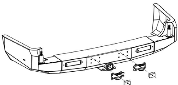
Install the lock supports using the provided hardware. ( If option wheel or jerrycan )
